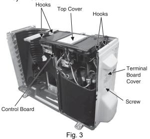
5 Remove the Control Board as follows:
