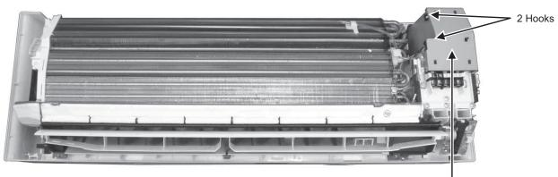
4. Remove the control board cover by releasing 2 hooks.
