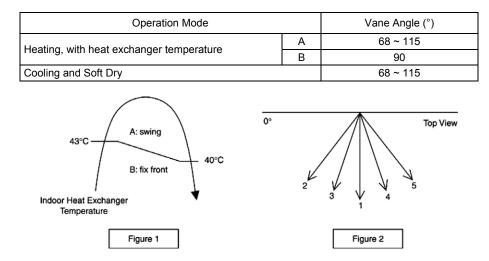
2 Manual horizontal airflow direction can be set using remote control; the angles of the vane are as stated below and the positions of the vane are as Figure 2 above.
