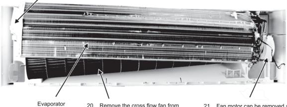
20. Remove the cross flow fan from the unit by pulling it to the left and downward.
