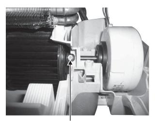
16. Remove the screw that holds the cross flow fan and the fan motor shaft.
