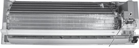
Remove the Control Board cover by releasing the hook.
