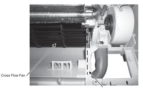
Reminder: To reinstall the cross flow fan, ensure cross flow fan is in line as shown in figure 10.
