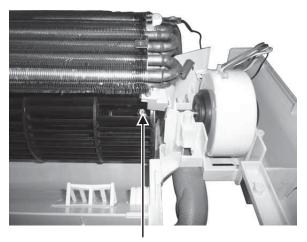
13. Remove the screw that holding the cross flow fan and fan motor shaft.
